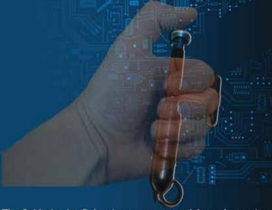
The Guidosimplex Pulsar is a compact standalone electronic accelerator that can be used in either hand; accommodating for driving with both hands on the steering wheel
