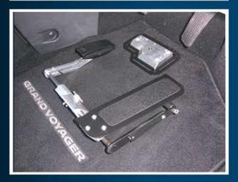
The fully adjustable PME Left Foot Accelerator is an adaptive driving control that assists drivers with impaired right leg function.
