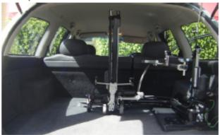
As it occupies very little space, the ABI Loader can be installed behind the rear seats in even relatively small cars like hatchbacks and compacts.
